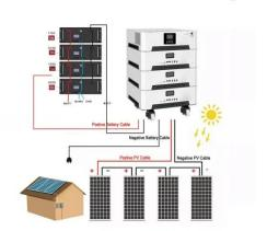
The Grid-tied solar inverters, otherwise known as on-grid or grid-connected systems, are the most common and straightforward type of solar installation. These systems are directly connected to
