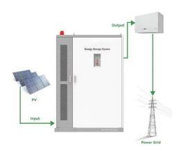
Jun 13, 2025 · Discover how energy storage inverters enhance solar systems by converting DC to AC power, storing excess energy, and offering backup during outages. Boost efficiency today!
