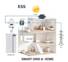
All-in-One Energy Solution: This comprehensive system integrates a 5kW hybrid inverter and 5kWh capacity lithium-ion battery, providing a seamless and efficient energy storage solution ...
