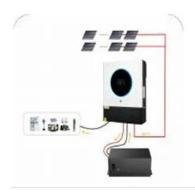
device that converts direct current (DC) energy from a 12V battery into alternating current (AC) energy. This allows the use of battery power for ...
